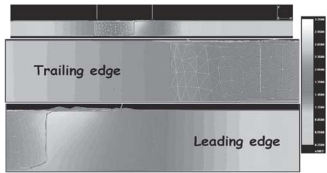
Fig. 3 Temperature distribution over the XY-plane
